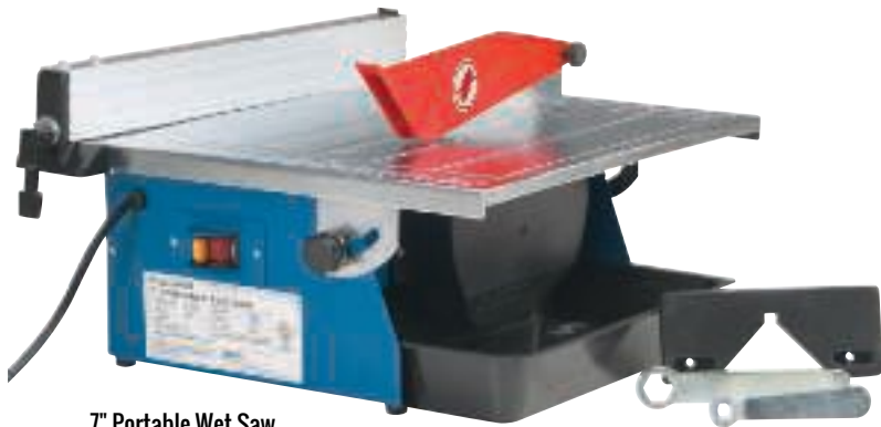
7" Portable Wet Saw • High output, direct drive, 1/3 HP motor, 120V/60Hz, speed 3,400 RPM • Adjustable cutting table raises with set positions enabling 15°, 30°, 45°, and 60° precision cuts • Equipped with 7" continuous rim diamond blade • Also accepts 6" blades 286265 $99.99
