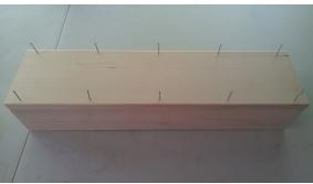
2. Set the bottom piece on top of the two 1x4 side pieces, lining them up so the edges are flush.
