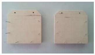
4. Predrill holes for the pulls near the top of the end pieces and start 6 nails in each.
