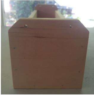
5. Line up the end pieces with the sides and bottom and drive all of the nails.
