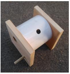
2. Line up the 1x6 front and back pieces with the 4" PVC and insert the %" dowel through the front piece and through the back until it's flush. The front piece has a 1 %" hole centered 2" in from each edge and a %" hole centered 1 ½" in from each edge. The back piece has a %" hole in the center and four %" holes centered 1 ½" in from each edge to form an X.
