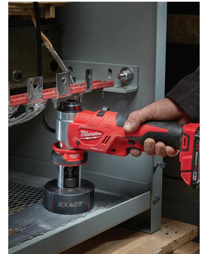
**M18™ FORCE LOGIC™ 10 Ton Knockout Tool Kit**
